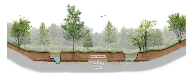
Pre-restoration conditions depict a channelized waterway with unstable, high banks of legacy sediment along waterways. During a typical rain event, soils erode from these banks and water velocity increases. In an extreme event, damage and flooding can be severe.
