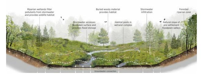
Post-restoration conditions depict a gradual slope to a widened floodplain. During a rain event, water can access the floodplain and its velocity is slowed. Water soaks in place and recharge the groundwater storage. In an extreme event, it exceeds capacity and flooding occurs.
